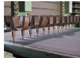
Resistance welding of cathode mesh
